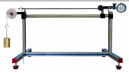
The **Portal Frame Unit Model KSM-052** is designed to measure the deflection at the load point of a rectangular portal frame subjected to both horizontal and vertical loads. The system consists of a frame fixed to a rigid base, with loads applied via mass hangers and a range of weights. Horizontal and vertical deflections of the frame are measured using dial gauges.
